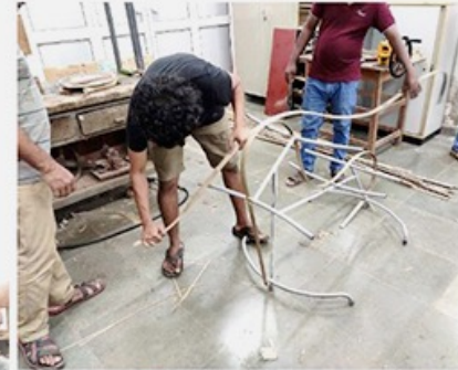
Bent slivers putting on frame
